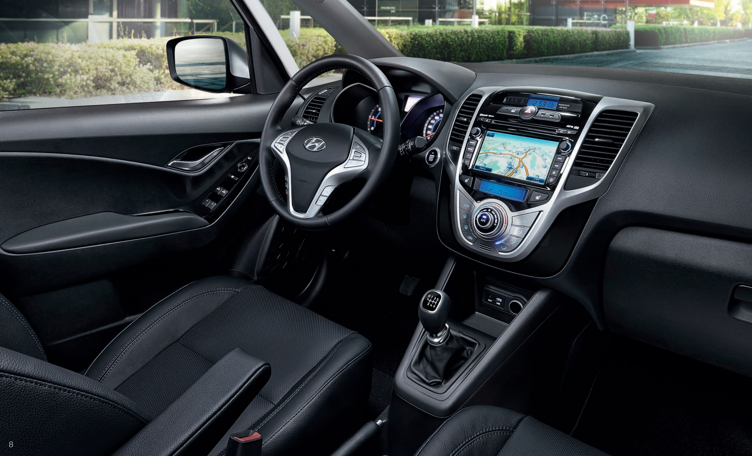
New generation audio and navigation system. The new audio system includes iPod connectivity, integrated My Music storage (1 GB) and AUX and USB ports. The navigation system has a 6.5" TFT colour touch screen that also functions as the display for the integrated rear view camera.
